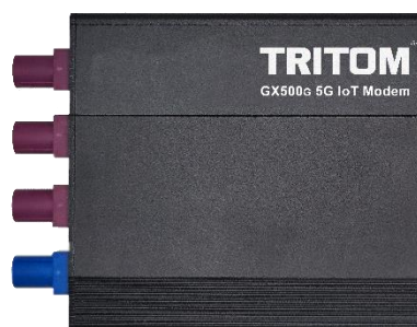
FAKRA connector for external antenna Option: SMA connector
